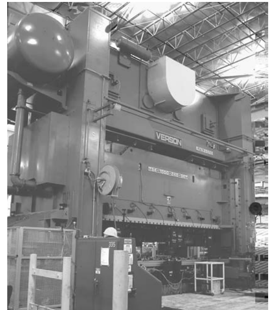
Installation of a 1500 ton press on MXL elastomer isolators.
