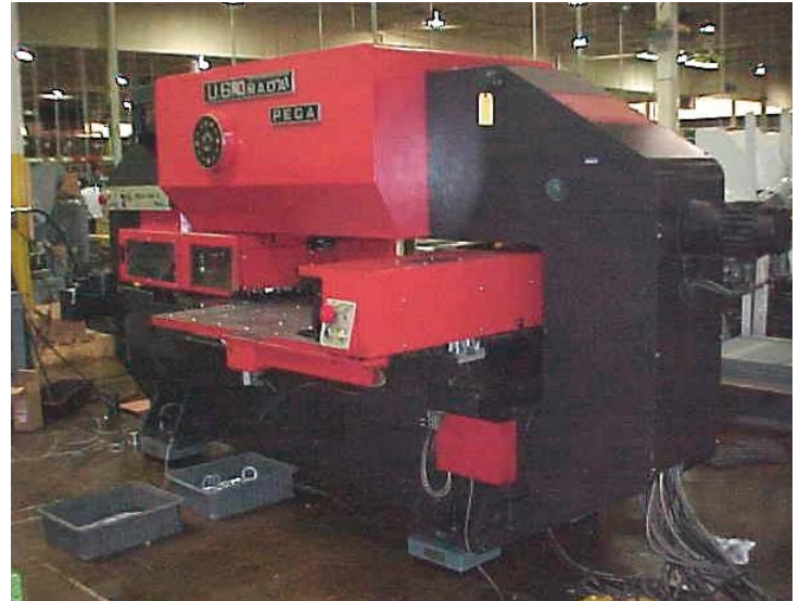
U.S. Amada Turret Punch Press on Vibro/Dynamics 10M1200H 1.25H8 Micro/Level® Isolators
